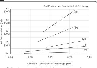
The Kdr value may be used to calculate discharge capacity in accordance with ISO 4126. We recommend contacting us with system details to confirm suitability
