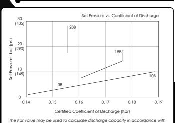
ISO 4126. We recommend contacting us with system details to confirm suitability.
