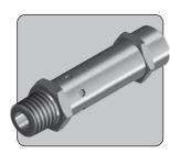
The \$50 is a vent to atmosphere safety relief valve. Designed with an elastomeric seat seal the valve combines excellent leakage performance with a nigh discharge flow capacity from its pop-open characteristic.
