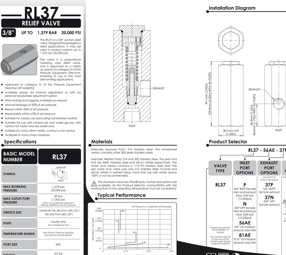
Certified Coefficient of Discharge (kdr) The kdr value may be used to calculate discharge capacity in accordance with ISO 4126. We recommend contacting us with system details to confirm suitability
