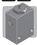
The PCFR50 is a pressure compensated flow control valve. Unlike a standard metering valve, the PCFR50 provides a relatively constant flow in one direction, regardless of the pressure differential across the valve, and is ideal for providing constant speed control of functions that have variable loads.
